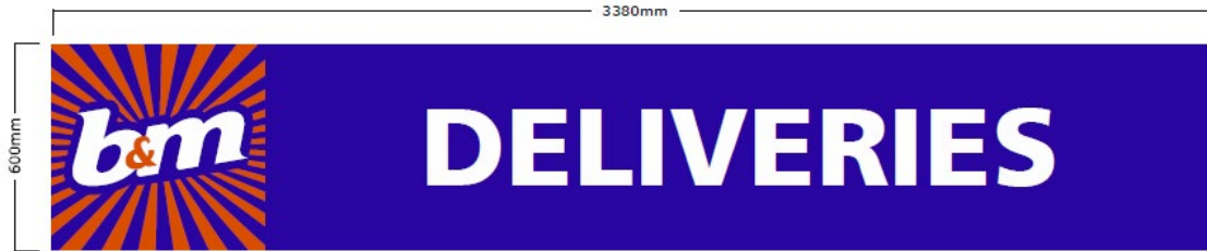
1No. Digitally printed and laminated 3mm flat Dibond panel, printed into standard colours
