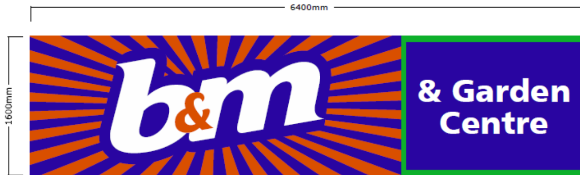
1No. Non illuminated flex face fascia frame complete with digitally printed/laminated flex face skin
