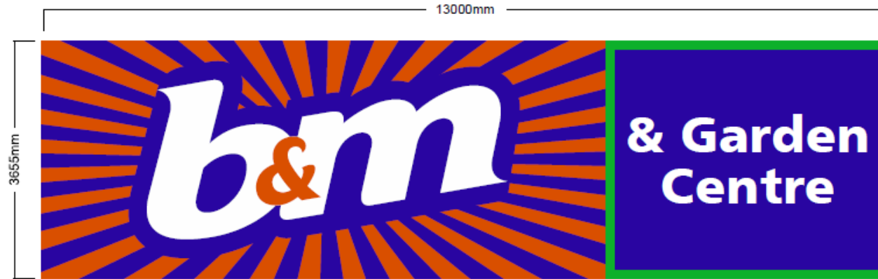
1No. Internally LED illuminated flex face box sign complete with digitally printed and laminated flex face PVC skin and bird spikes macroart
